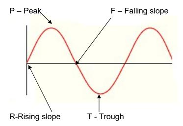
This enables full flexibility on the testing conditions. The slowest response time for the RCD will be if the testing is started on either R or F. This will be the worst case situation and is the recommended testing point for testing the trip time. The slope selection does not apply for the Type I Medical tests the starting point is selected randomly as per AS3003.
